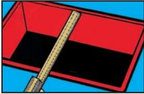
**1** Measure the opening to ensure that its size conforms with tolerance standards 120,5 mm ( $\pm 0,5$ ).
