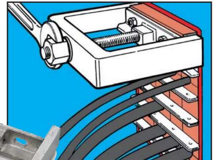
**3** Tighten the bolt on the puller and the endpacking slides out.
