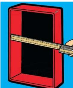
Measure the opening to ensure that its size conforms with tolerance standards  $120,5\text{ mm } (\pm 0,5)$ .
