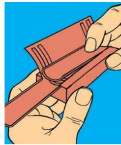
Place sheet into centre slot and affix it with the unique locking device.
