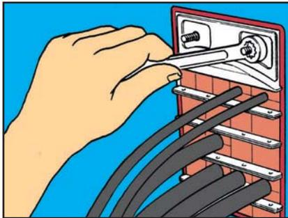
**2** Attach the endpacking puller to the bolts with the nuts.
