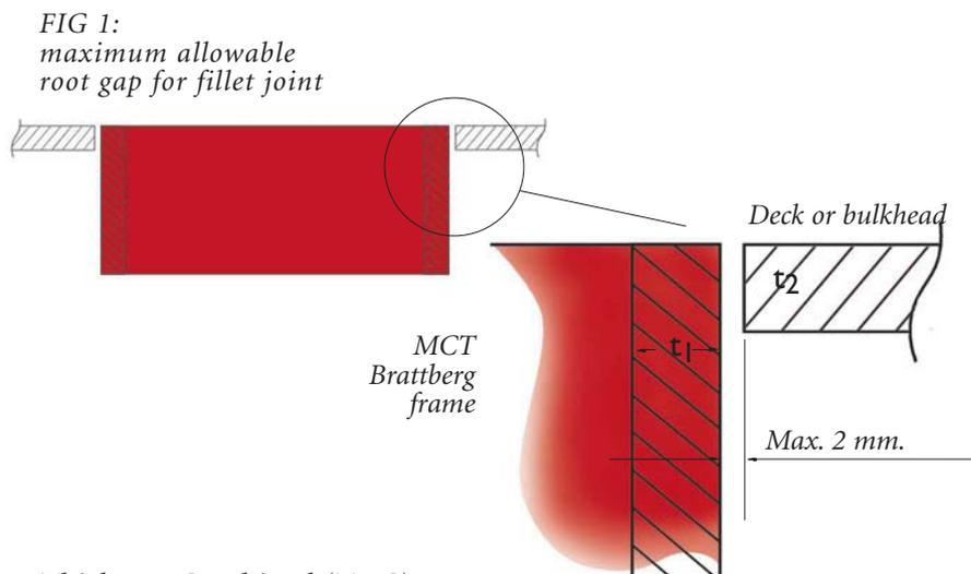
Thickness Combined (THC) =  $t_1 + t_2$
