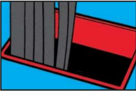
**5** Pack the last row, then tighten the bolt on the compression plate counter-clockwise until there is 32 mm of space between the top of the plate and the frame or enough to fit the endpacking tongue around the bolt.
