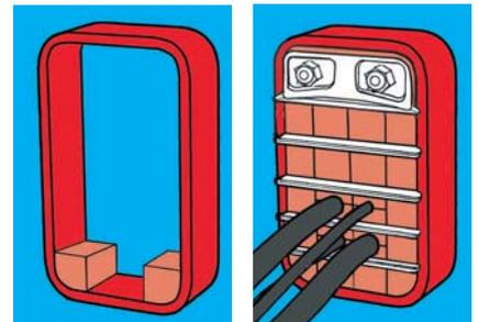
Begin packing with the special corner blocks. Insert endpacking STG with the tongue around the compression bolt. Tighten the nuts on the endpacking to compress and complete the seal. Approximately 12 mm of thread should protrude on each bolt.
