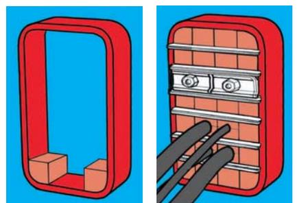
Begin packing using the special corner blocks. Place the PTG Presswedge anywhere, except at the top or bottom.
