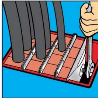
**4** Insert the outer blocks first (A, B, C etc.). Then insert the remaining blocks. Note. The block A should be turned 90°, as shown in the picture.
