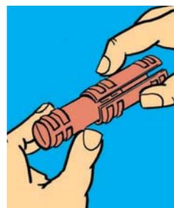
The centre plug is a snug fit for any pre-selected AddBlock since its diameter is adjustable - all thanks to the wraparound casing.
