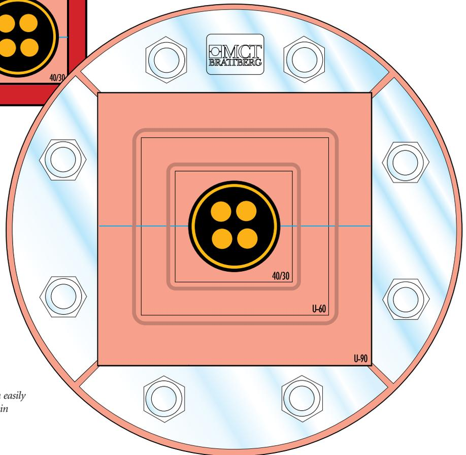
With U-Blocks, you can easily center the cable or pipe in your RGP installation.
