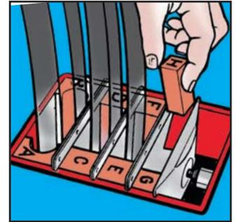
**6** Insert endpacking STG with the tongue around the compression bolt. Tighten the nuts on the endpacking to compress and complete the seal. Approximately 12 mm of thread should protrude on each bolt.
