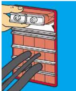
**5** Fit first the PTG presswedge at top of the frame. Insert then the last row of blocks.
