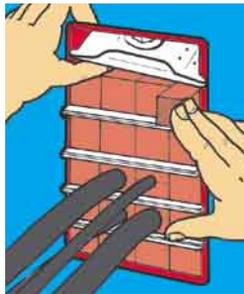
**5-6** Insert the last row of blocks. Tighten the bolt until there is 32 mm between the top of the plate and the inside of the frame.
