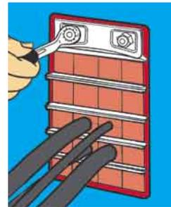
**7** Insert endpacking STG with the tongue around the compression bolt. Tighten the nuts on the endpacking to compress and complete the seal. Approximately 12 mm of thread should protrude on each bolt.
