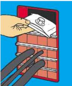
**4** Insert the compression plate in the frame before the last row of blocks.
