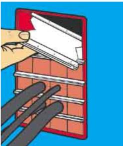
**4** Insert the last two stayplates in the frame before the last row of blocks.
